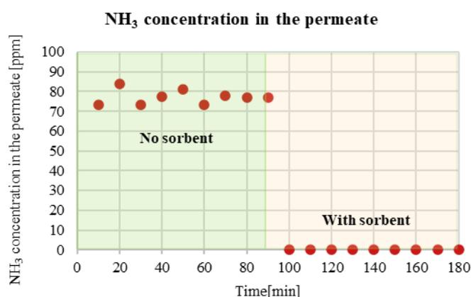
**Figure 4. Removing the ammonia content in the permeate of the ammonia decomposition membrane reactor using a sorbent. Experimental conditions:  $T = 400\text{ }^{\circ}\text{C}$ ,  $P_{\text{retentate}} = 3\text{ bar}$ ,  $P_{\text{permeate}} = 1\text{ bar}$ .**
