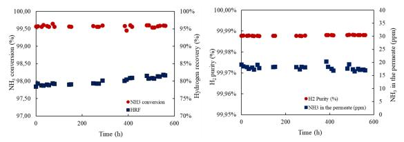
Figure 2. Long term ammonia decomposition test in the membrane reactor. Experimental conditions: T= 450 °C,  $P_{retentate}= 3$  bar,  $P_{permeate}=$  atmospheric, Feed= 0.5  $L_N$ /min NH<sub>3</sub> (see reference 2 in peer review articles section).
