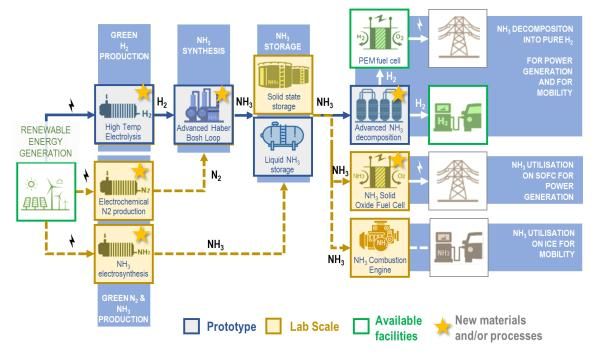
Figure 1. Power-to-ammonia-to-usage value chain in ARENHA
